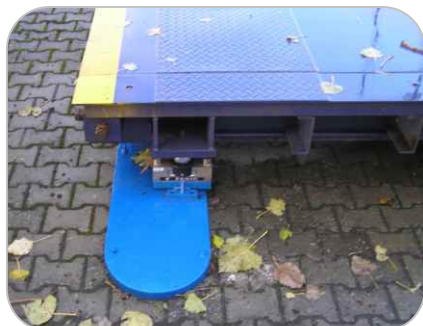
Installation of an HM9B load cell at a platform
